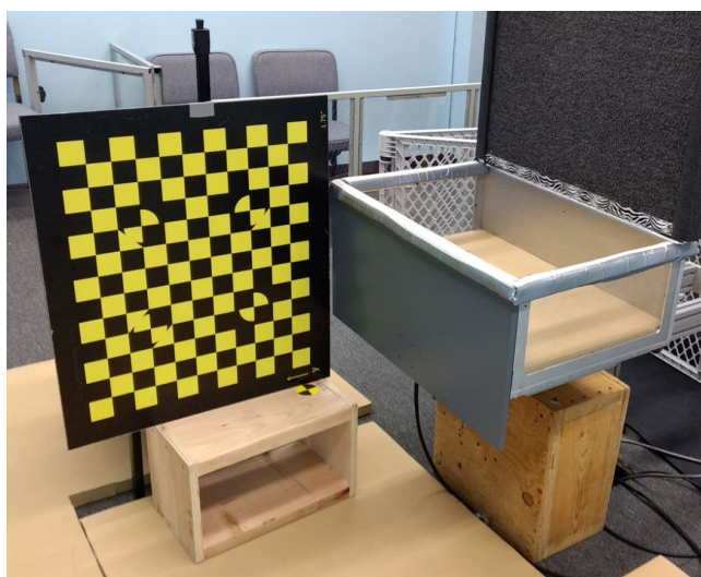
Figure 12. Camera calibration grid set up for the side-view webcam.
