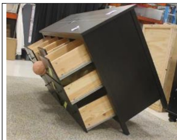
Figure 48. ES staff reenactment of incident. Dresser propped up by the lower drawers with dummy in the middle right drawer (left).
