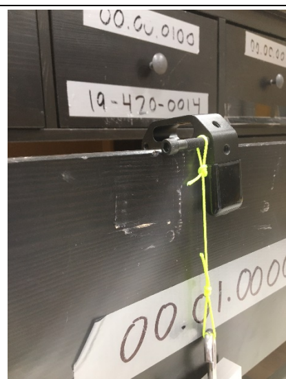
Figure 130. Force gauge attachment
