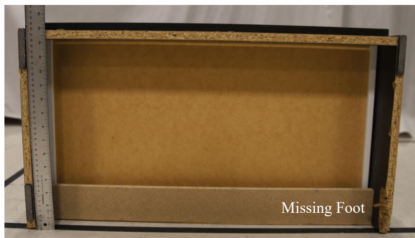
Figure 23. The bottom of the CSU with 1 missing foot.
