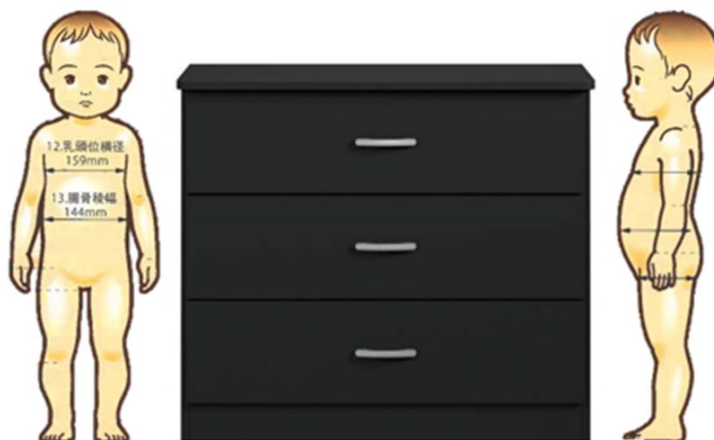
Figure 18. Scaled drawing of the 32 in. 2-year-old child with 27.5 in. dresser.
