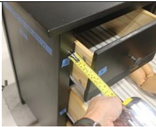
Figure 57. Dresser unstable (tip over occurs), 6 drawers open, 7th drawer partially open. The dresser becomes tips over when 6 of 8 drawers are fully open (Figure 27), the 7th drawer is extended/partially opened 3.25 inches, and the 8th drawer remains closed.
