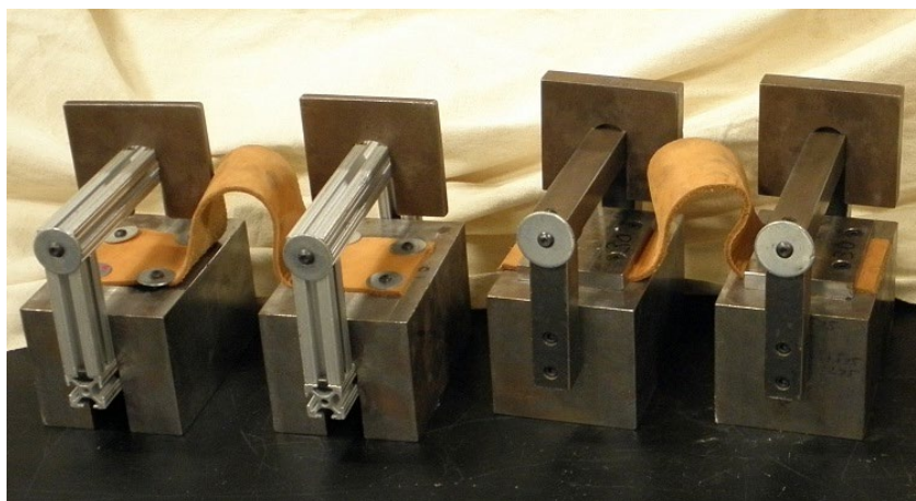
Figure 3. The test weights staff used to determine tip weight. The 30-pound base test weight, used for 30-59 pounds, is shown on the left with 2 pounds of additional weight added (1 pound on each side). The 60-pound base test weight, used for 60-134 pounds, is shown on the right with 5 pounds of additional weight added (2.5 pounds on each side).
