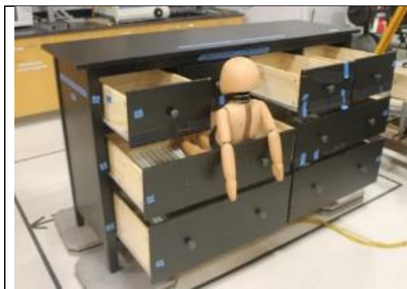
Figure 66. Weighted dummy (30 pounds) in the middle drawer. Six (6) drawers are fully opened/extended, the 7th top left drawer is partially opened/extended to 9 inches, and the 8 th drawer is closed.
