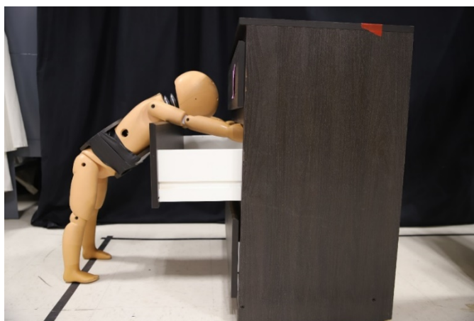
Figure 26. A dummy weighing approximately 30 lbs. is shown balanced on the front of the middle drawer of the product. Pushing the dummy forward slightly caused the product to tip.
