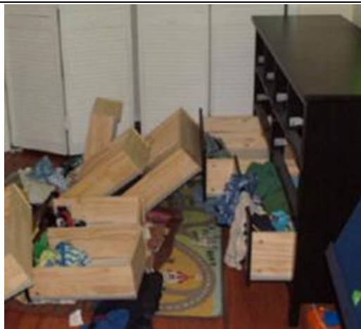
Figure 50. Incident scene show one filled bottom drawer and various partially filled drawers (left). ES staff filled the drawers with 10 pounds of clothing to recreate the incident scene.
