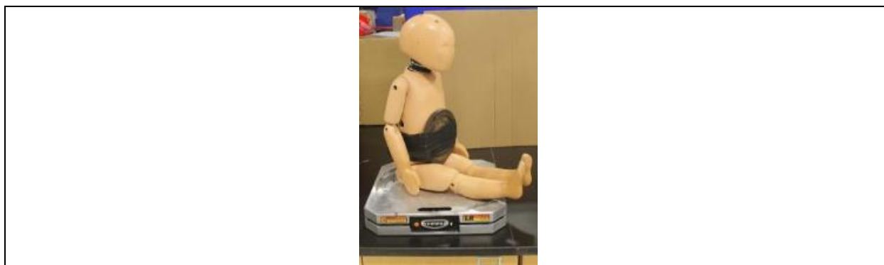
Figure 55. 18-month-old CRABI crash test dummy with added weight, such that total weight = 30 pounds (left).
