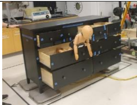
Figure 56. Dresser in the tip over condition-dummy leaning forward, (ES staff holding dresser from falling over) 6 of 8 drawers fully open, one top drawer partially open (7th drawer), one top drawer closed (8th drawer). All drawers empty (no weight). Weighted dummy (30 pounds) leaning over front edge of drawer.
