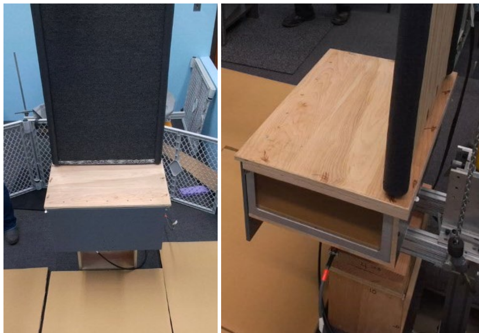
Figure 8. Photos of the table condition from two perspectives, showing the flat wood tabletop added to the box frame.
