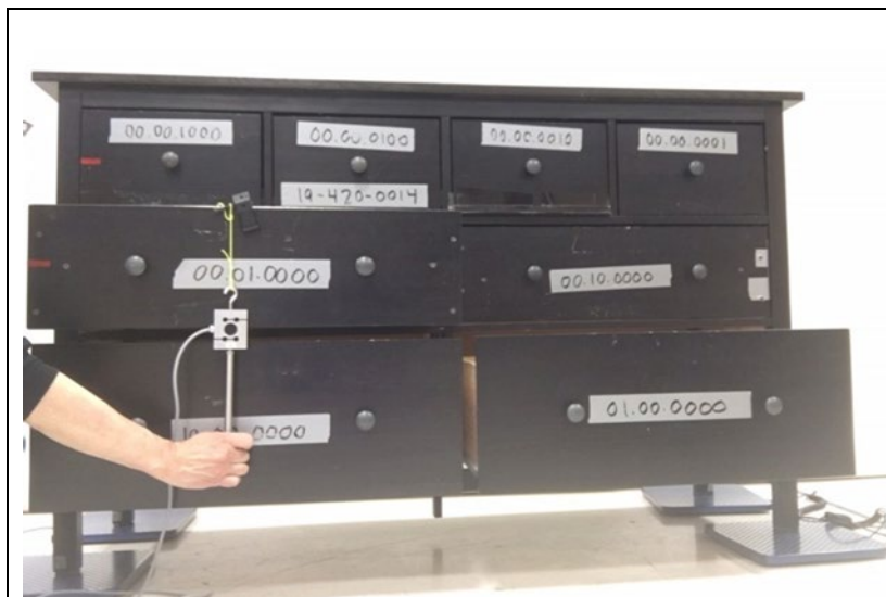
Figure 129. Force gauge on drawer
