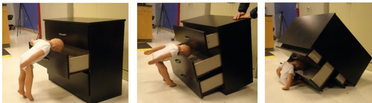
Figure 19. The illustration of the hazard scenario described above shows a doll with a height of about 32 inches, the height of the victim.
