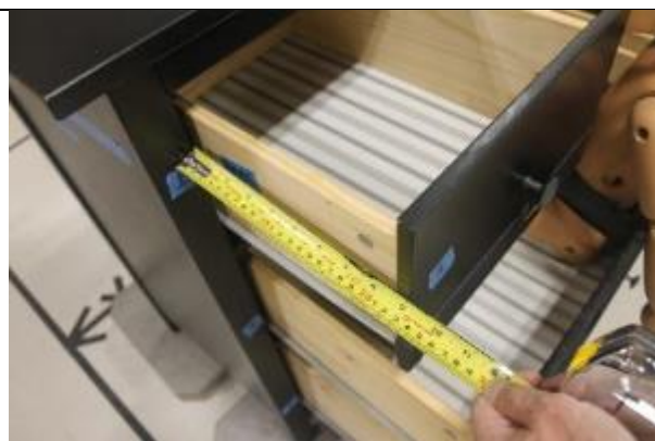
Figure 67. Dresser is balanced on front legs when the top 7 th drawer is pulled out 9 inches. If the 7 th drawer is then fully opened, the dresser tips over.
