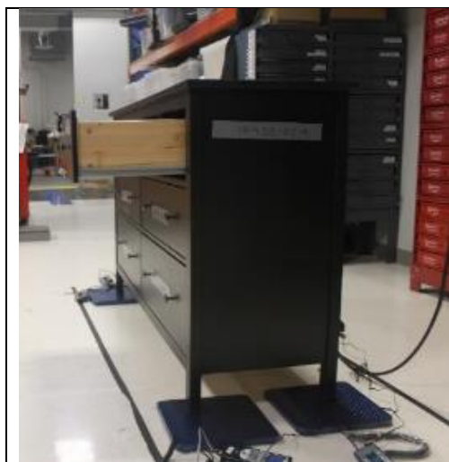
Figure 101. Sample 19-420-0014 (weight = 122 pounds), two (2) top drawers open.
